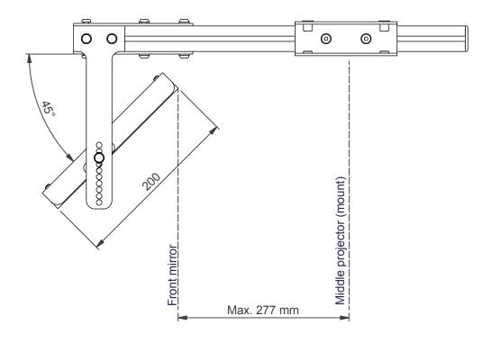
Max. lens offset 85 mm. Mirrorsize 200 X 200 mm. NOTE: All dimensions are ±..., in mm and subject to change © COPYRIGHT AUDIPACK **AUDIPACK**
