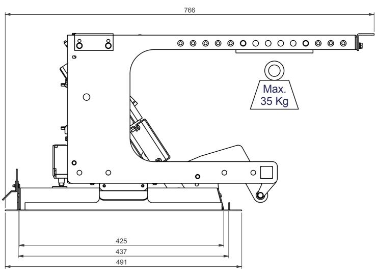
Suitable for projectors up to 150 mm body thickness Suitable for wide screen 16:9 - 16:10 projectors Max. projector height 150 mm Max. product weight 35 Kg
