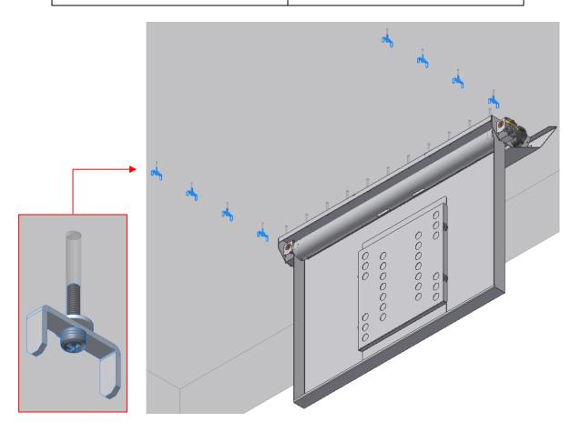
**7.** To join the cover plates use the fixing plates.
