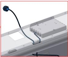
**13.** Install the TV. Position the magnets so the insert in the adjustable plate with holes. This plate is adjustable in height to line-out the TV.
