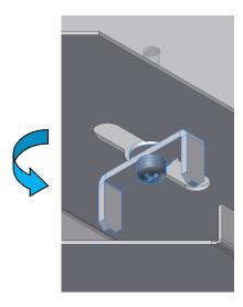
**9.** Position the inner cover plates inside the lift finishing.
