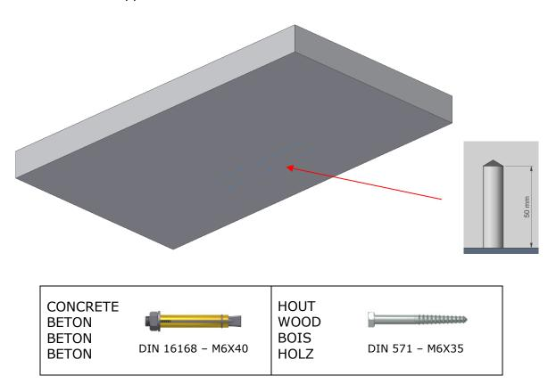
**2.** Position the lift and mount it with the M6 bolts.
