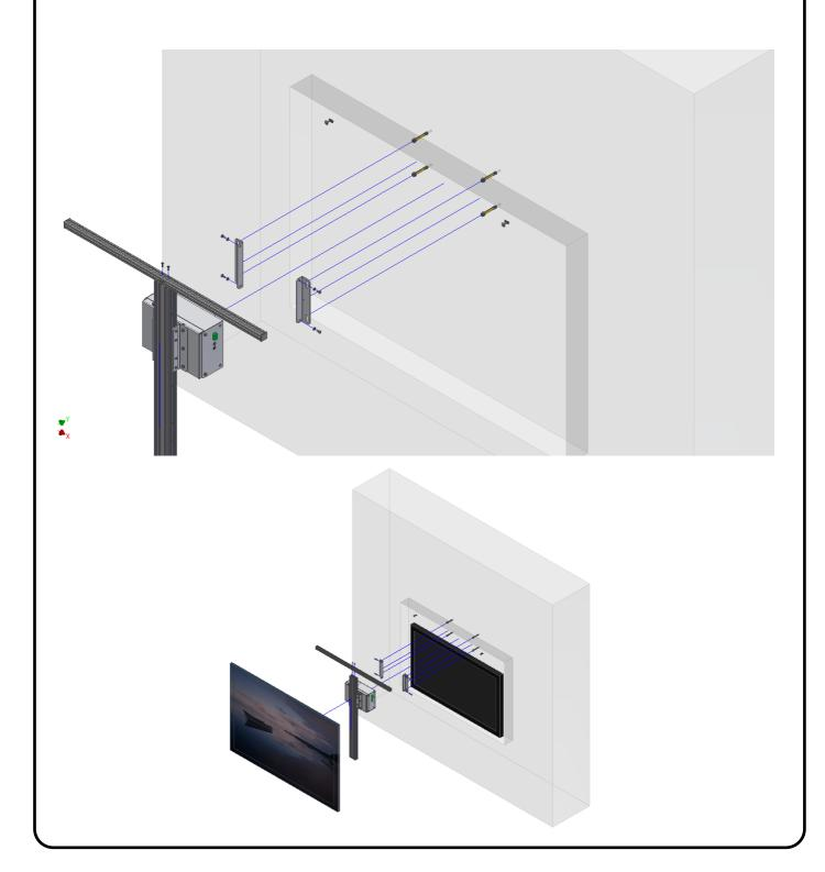
**2.** Install the AWL lift using all srews in the wall possible. By losening the bottom screw it is possible to slightly pivot the unit. Fasten all bolts well.
