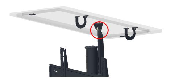
**7.** When provided, install the monitor cables in the cable guidance of the lift.
