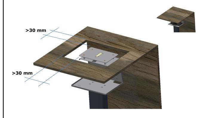
2. When the lift is installed the finishing panel can be installed. Mount the panel to the magnet. Use the attached drawing for accurate positioning.
