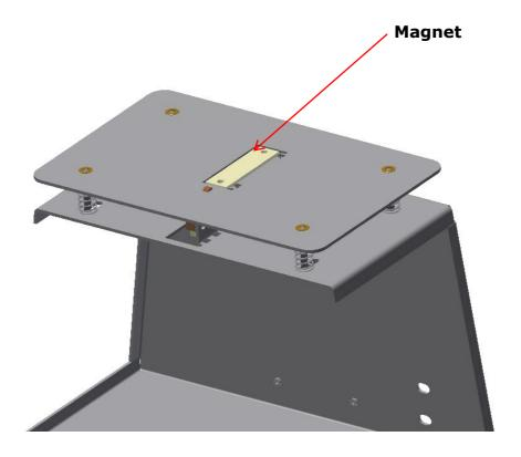
3. When the panel is installed, the height position can be adjusted with the scews in the springs. The screws allow only a small adjustment height. Level the system when more adjustment is needed.
