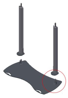
**3.** Install the top part with the lifting head. Be sure to grip the handle and the side of the colums. Do not lift at the lifting head!!
