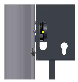
At the front of the lifting head coloured knobs are visible. With an alan key the positions can be set by adjusting their position.
