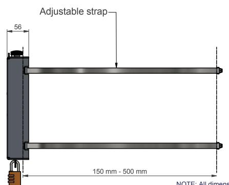
Suitable for columns from Min. Ø150 mm up to Max. 500 mm
