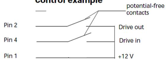
When the system must be connected or activated with an external control system, use the above listed option:
